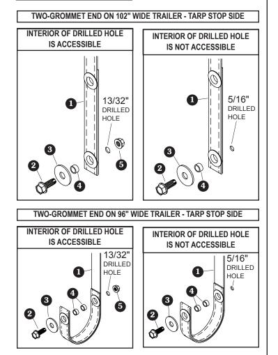
screws 20, washers 30, spacers 30 and nuts 50. If drilled hole is not accessible from inside of trailer and wall thickness is at least 3/16", fasten cord with screws 2, washers • and spacers •. **ONE-GROMMET END - LATCHPLATE SIDE** INTERIOR OF DRILLED HOLE INTERIOR OF DRILLED HOLE **IS ACCESSIBLE**
