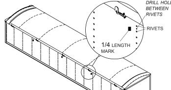
STEP 3: Roll tarp toward latchplate side and let roll tube hang at its lowest point. On latchplate side, locate row of rivets directly across trailer from selected row of rivets on tarp stop side. Drill hole between two rivets, just below lower edge of tarp.
