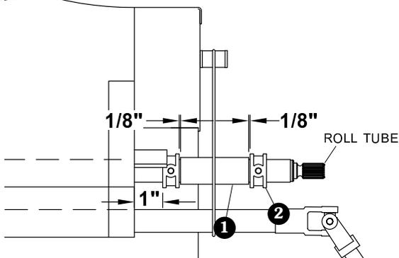
**STEP 3:** Fasten bearing rings 2 to roll tube with screws 3. Refasten U-joint and crank arm to roll tube with wire lock pin.
