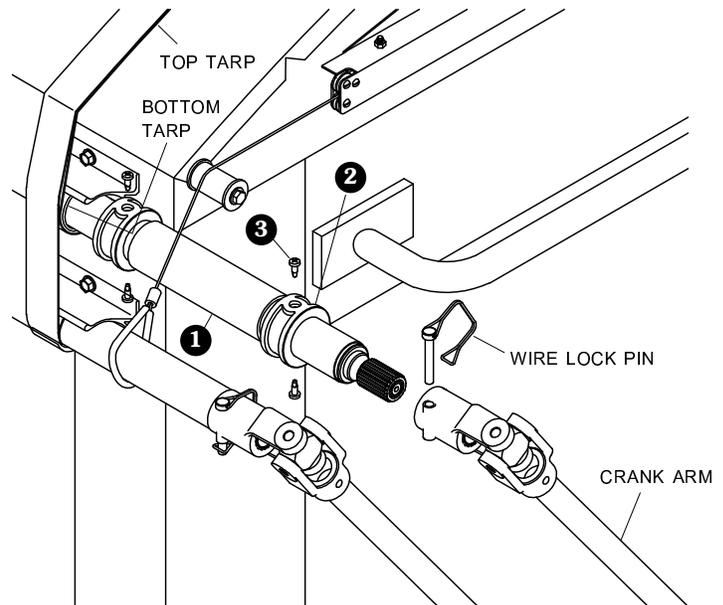
**NOTE:** Shorten cable roller 1 if needed to achieve correct distance for roll tube to extend past rear of box.
