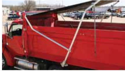
ARM-MATIC™ TENSION ARM KIT P/N 1120129 - For 10' Arms P/N 1120130 - For 12' Arms P/N 1120131 - For 14' Arms
