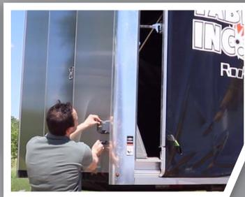
Release the tarp tension by rotating the safety lever on the headboard and pressing the OPEN button.
