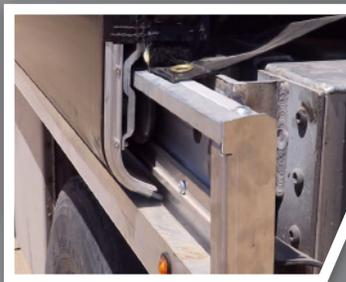
Push tarp system/bows to the front or back of the trailer, sliding on the TiteTrax™ track system.
