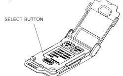
STEP 3: Put receiver into pair mode. On receiver, press and hold simultaneously both *Open* and *Close* buttons on receiver. After three seconds, you will hear buzzer beep. Release buttons. Receiver is now in pair mode.
