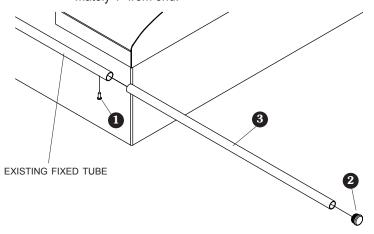
STEP 4: Using new self-tapping screw ①, secure tarp and fixed reinforcement tube using existing hole in fixed tube.
