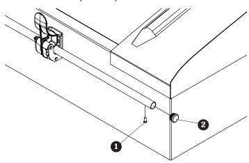
STEP 3: Place fixed tube reinforcement **③** in fixed tube approximately 1" from end.
