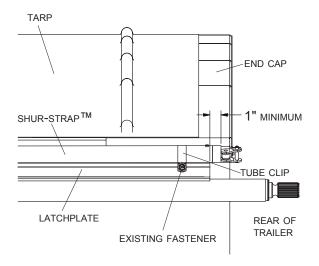
**NOTE:** If rear of trailer is free of obstacles, return may be mounted past face of end cap, allowing strap to float freely beyond trailer.
