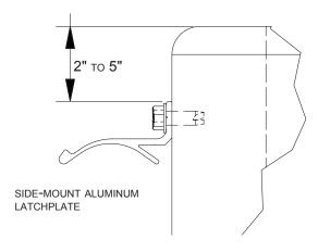
**STEP 2:** Latchplate should extend past tarp a minimum 1" at rear of tarp. If an aluminum end cap or combo cap is installed, at least 2" of end cap must be visible.
