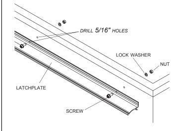
STEP 5: Using the same mounting fasteners in latchplate, attach Shur-Strap™ using tube clips. Extend Shur-Strap™ a minimum of 1" past latchplate.
