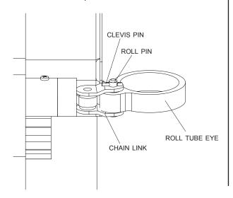
STEP 7: Roll tarp closed. Let tarp and roll tube hang down. Slide retaining collars and roll tube eye onto roll tube at rear of trailer. Align roll tube eye with strap. Space retaining rings about 1/8" to 1/4" from side of roll tube eye. Tighten self-tapping screws to secure each retaining collar.
