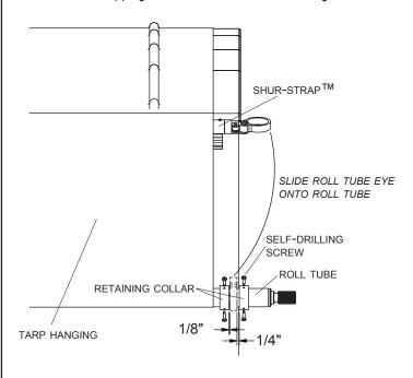
**STEP 8:** Roll tarp open and closed to make sure roll tube returns correctly, making sure strap does not come in contact with any sharp edges.
