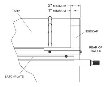
**STEP 3:** Mark hole locations on latchplate about every 2' apart, with holes no more than 6" from edge.
