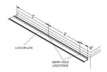
STEP 4: Drill 5/16" pilot holes through latchplate and box. Fasten with screws, lock washer and nuts.
