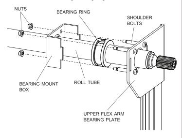
STEP 2: Turn bearing ring slightly to avoid using existing holes, drill two 3/16" holes and fasten rivets.
