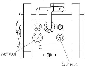
**STEP 2:** Install light to TrapAdapt<sup>™</sup> cart. Secure with lock washer and nut.
