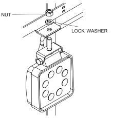
PO BOX 713 **2309** SHUR-LOK STREET YANKTON, SOUTH DAKOTA 57078-0713 PH. 1-800-474-8756 **FAX 605-665-0501**  STEP 3: Route LiteALL<sup>™</sup> wire along brace and down cart leg. Insert ends of wire through 7/8" hole and secure dome nut in hole using 1/2" NPT lock nut **③**.
