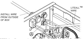
**STEP 4:** Remove slack from wire using cable ties ③ securing wire to light mounting bar and cart down tube.
