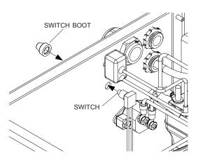
STEP 7: Plug male quick-disconnect into female quick-disconnect.
