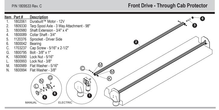
Before drilling holes in box, make sure there is enough room for tarp to roll up around tarp axle. Measure box and compare measurements with those shown.
