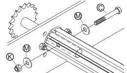
STEP 10A: Electric system. Slide flange bearing over stub shaft and fasten to outside of cab protector with bolts ☉, washers ℑ and nuts ❶. Tighten set bolts on bearing.
