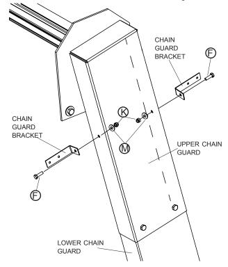
**STEP 10:** Secure chain guard brackets to truck box using sheet metal screws **O**.
