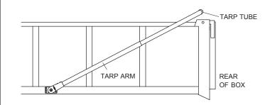
STEP 7: Drill 5/16" hole through both arms approximately 3" lower on lower arm. Attach with cap screw ⊙, flat washer ⊙ and lock nut ③.
