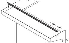
**STEP 7:** Drill 5/16" hole 5/8" in from cut end of tarp axle, aligning hole as shown.
