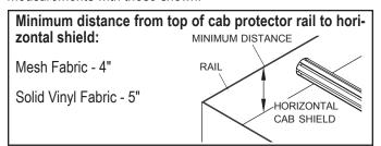
**STEP 1:** Determine tarp axle mounting location on cab protector. Location must keep spring-loaded arms from interfering with cab doors and exhaust stacks. Arms must not interfere with loading process.
