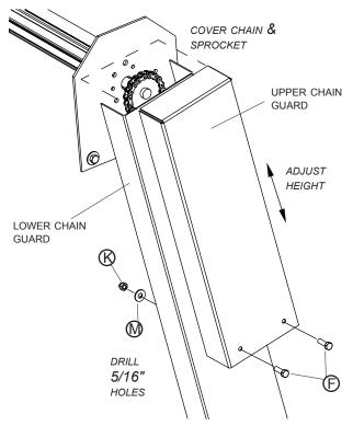
STEP 9: Attach chain guard brackets near top of upper chain guard. Mark and drill 5/16" holes through upper chain guard for mounting. Use 5/16" bolt <sup>①</sup>, washers <sup>①</sup> and lock nuts <sup>③</sup> to secure bracket to chain guard.
