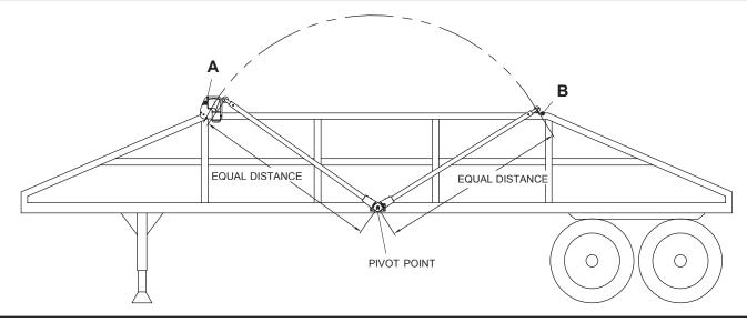
NOTE: Tapered, wedged, rounded or sloped trailers may require additional bracketry to offset and square arms with trailer.
