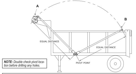
**NOTE:** To determine pivot point on opposite side of box, first make sure box is square. Transfer measurement from point A to pivot point over to opposite side of box.
