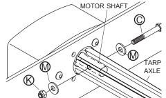
**STEP 9B: Manual system.** Fasten tarp axle to sprocket shaft with screw **(()**, washers **(()** and nut **(()**.
