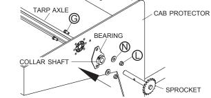
STEP 9A: Electric system. Fasten tarp axle to motor shaft with bolt ⊙, washers ⊙ and nut ③.
