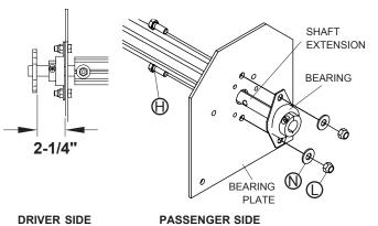
STEP 8: Tighten set screw on ball bearing.
