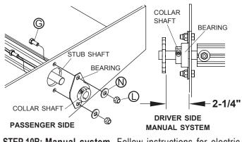
**STEP 10B: Manual system.** Follow instructions for electric system in step 10A. On driver side, adjust sprocket location as shown, then tighten all bearing fasteners and set screws.
