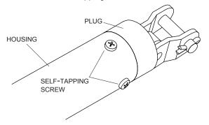
**STEP 2:** Remove spring assembly from housing.
