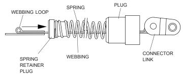
STEP 7: Insert spring pin through loop in webbing and cut off tail.
