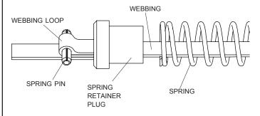
STEP 8: Re-install webbing and spring assembly into Shur-Strap™ housing. Secure with self-tapping screws.
