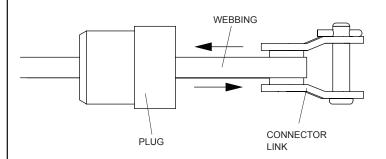
**STEP 6:** "Fish" new webbing through plug, spring and spring retainer plug.
