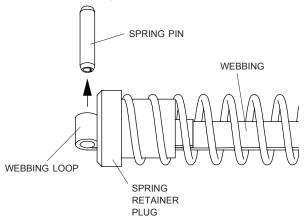
**STEP 4:** Pull webbing and connector link off spring.
