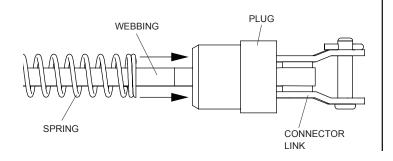
**STEP 5:** Remove plug from webbing and connector link.
