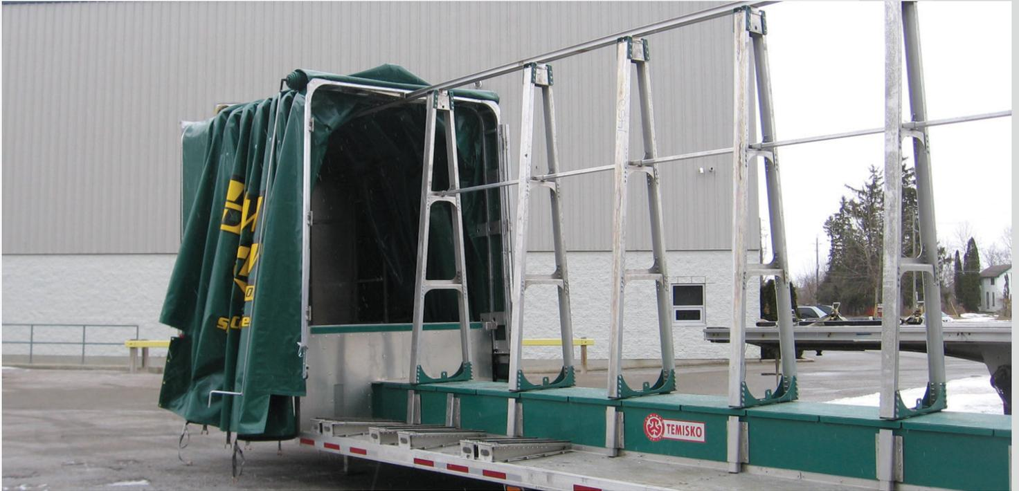
Glass-hauling systems are designed with a specialty all-aluminum headboard and unique monorail system that mounts on top of the A-frame and opens from the rear.
