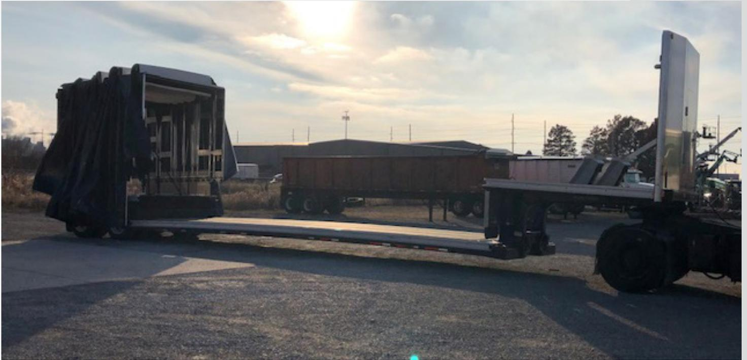
Lower deck bows come equipped with a triple set of wheels to transition to either front or rear raised decks. Drops must constitute a difference of 8 inches to completely transition system from front to rear.
