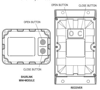
Option 2: Standard receiver boxes only: Remove six screws holding plastic cover on receiver box. Gently pull cover off, but do not disconnect any wires. Press and hold programming button next to red light. Red light will go solid. After three seconds, light will start blinking and buzzer will beep. Release button. Receiver is now in Pair Mode.
