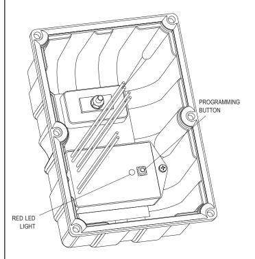
STEP 4: Put remote into pair mode. Pick up remote and press and hold simultaneously both *OPEN* and *CLOSE* buttons on remote. After three seconds, channel indicator light will go solid. Release buttons.
