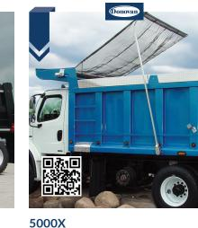
The most popular line of economical, yet dependable, front-to-rear tarp in a wide variety of models, by cab or ground-level manual crank or Durabuilt™ direct-drive motor.
