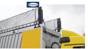
The Double-Flip<sup>™</sup> opens and closes in under 10 seconds! Simple to operate, easy to maintain and affordable. Designed to cover open-top transfer trailers with a hydraulic power gantry and tarp roller that operates off the trailer's hydraulics.
