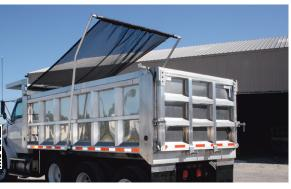
• Extruded Aluminum Roller Bar with Side Plates • Aluminum High-Gloss Pivot Arms - 1 PC. Aluminum • Assembled Housing - Standard for 38' and 41' Kits • High-Mount Compatible - Up to 23' Only
