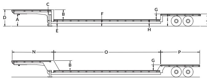
Use diagram below to help determine correct measurements for ordering. Trailer **MUST BE AIRED UP** and hooked to the truck or the fifth-wheel height set to 48" from the ground BEFORE taking measurements. Width of deck is from outside rub rail to outside rub rail. Additional information needed is noted on reverse side.
