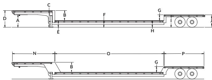
Use diagram below to help determine correct measurements for ordering. Trailer **MUST BE AIRED UP** and hooked to the truck or the fifth-wheel height set to 48" from the ground BEFORE taking measurements. Width of deck is from outside rub rail to outside rub rail. Additional information needed is noted on reverse side.
