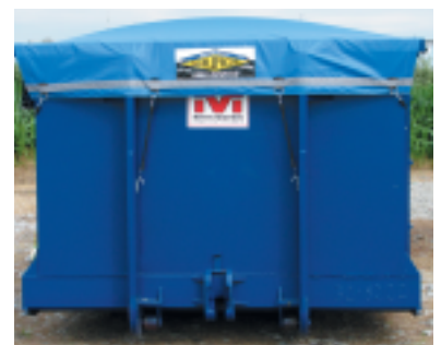
Top to bottom: PBR roll tarp cover equipped with offset tarp stops and crank arm storage; fabric end flap on PBR cover; and roll-off container fitted with a Shur-Lok®.
